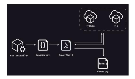
Looking inside the installer reveals the Custom Action that's responsible for initially running the JavaScript embedded inside the installer.
